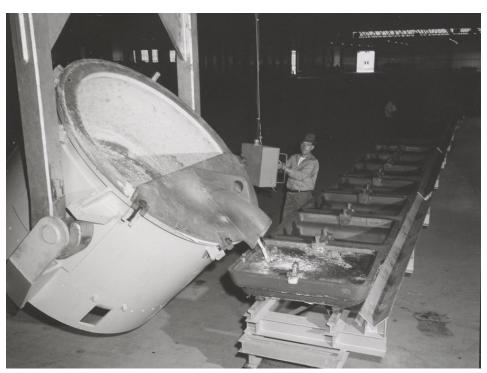
On June 10, 1960, the first smelting pot at Alcoa Warrick Operations was tapped and molten aluminum was poured into pig-style ingots.
